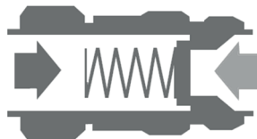
Reverse flow - valve closes
